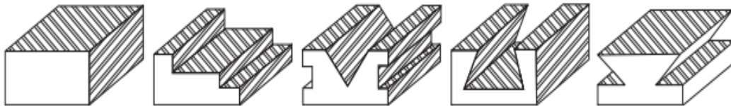
Fig. 6 Various components manufactured by planning/ shaping process
